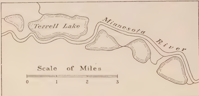
FIG. 113. — Shallow basins formed as a result of the building of natural levees along the stream are filled at flood time with water from the stream and from the sides of the valley. (Minneapolis topographic sheet, U. S. Geol. Surv.)
